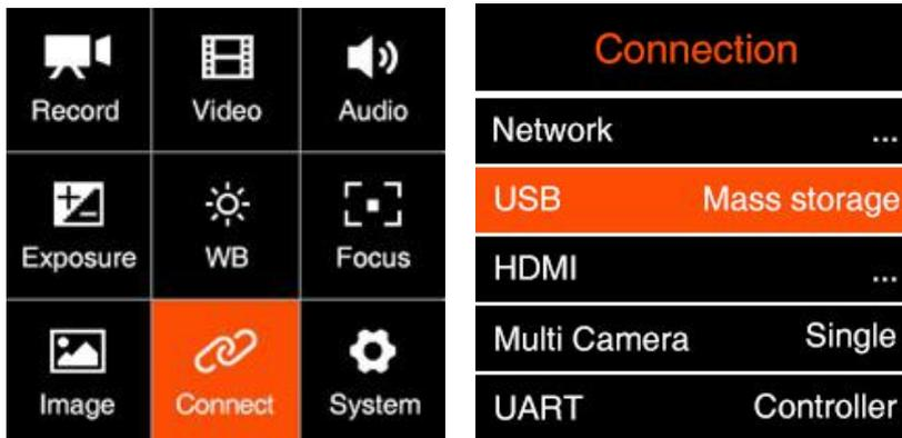
3. Connect the camera to a computer with a USB Type C cable, an “USB” icon would show up on LCD screen, then it’s connected successfully.
