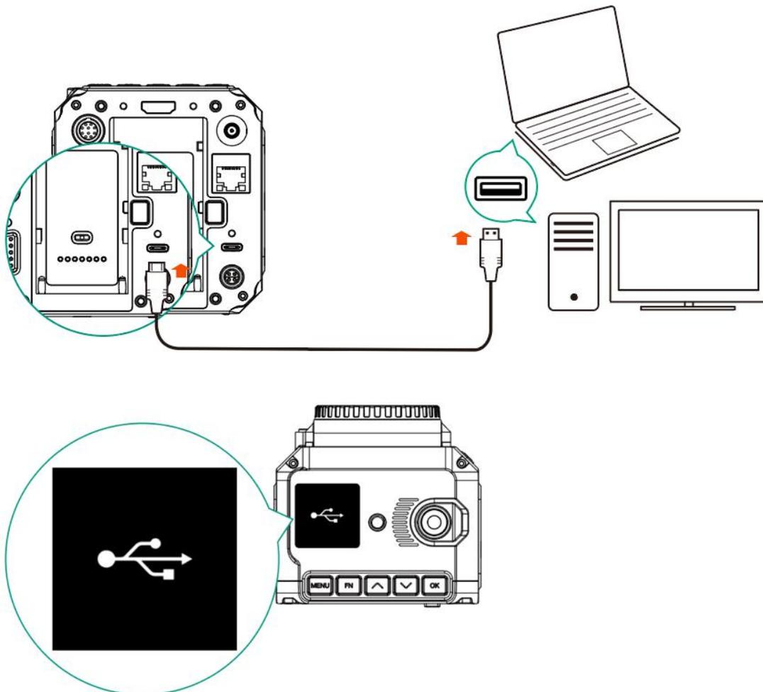
4. PC will detect the camera and shows it as external storage device. You can access & manage the files in the CFast card inside the camera.
