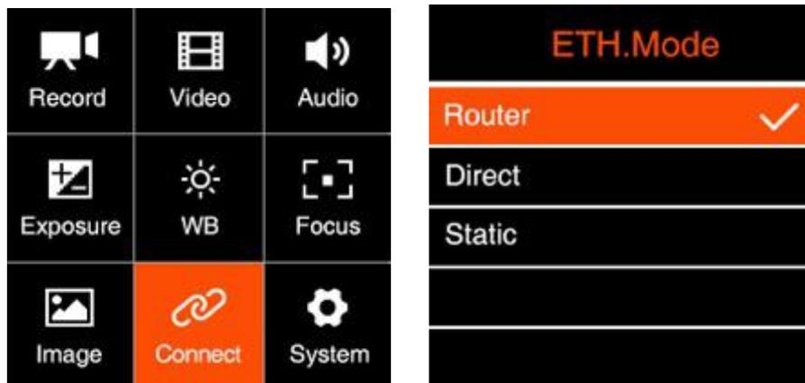
2. Connect the camera to a router with an Ethernet cable, then connect the router to the computer with Ethernet cable or Wi-Fi. (Note: Camera and PC should connect to the LAN port of router, not WAN port)
