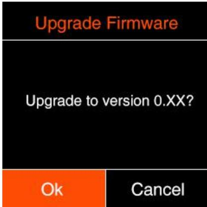
4. If the version of the **update.zip** file in CFast card is the same as or lower than the camera's one (to refresh or downgrade the firmware), there will be no pop-up message when the camera is powered on. Go to **Version** in **System** setting, press **OK** button and you will see the pop-up message for firmware update. Select "OK" and press **OK** button to update the firmware\*.
