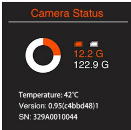
5. When the temperature exceeds 60°C (140°F), press the **Record** button to stop recording.
