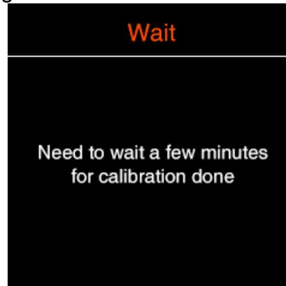
Note that the **Sensor Calibration** will take about 2 minutes, and **Hot Pixel Calibration** will take 5-30 minutes for Z CAM E2 and 5-10 minutes for Z CAM E2 Flagship series.
