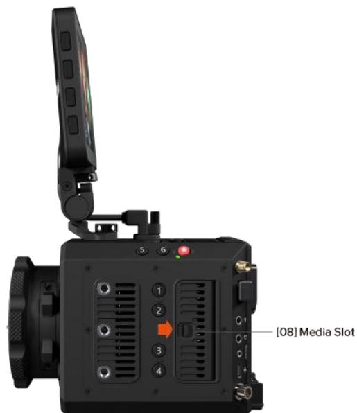
**Attention:** When using a CFast card (or ZBlade) on Z CAM E2-F6 Pro for the first time, please format it before recording (**System – Format Card**).
